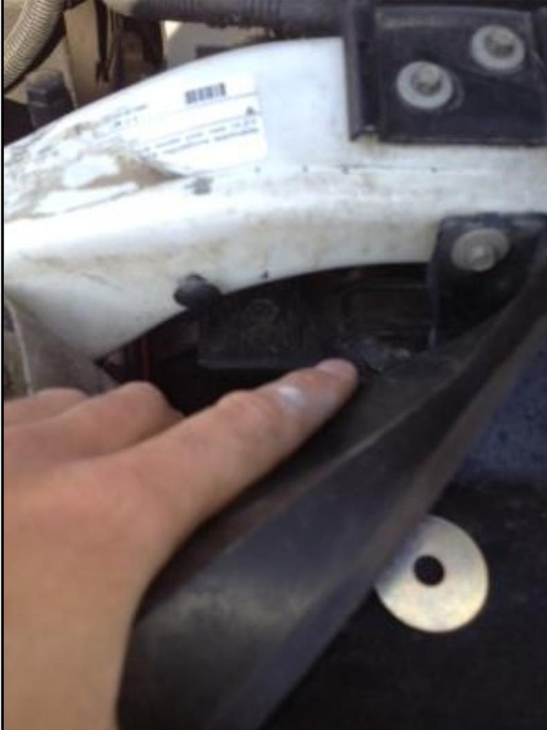
5. Place sleeve in bracket and Install 3/8x5" Bolt through Bracket and Sleeve as pictured.
