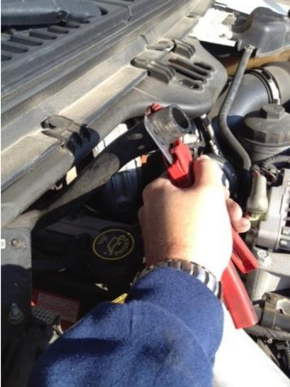
10. Install larger clamps on hose and install the machined tee after routing the hose to prevent chafing on sharp objects. Tighten Clamps.
