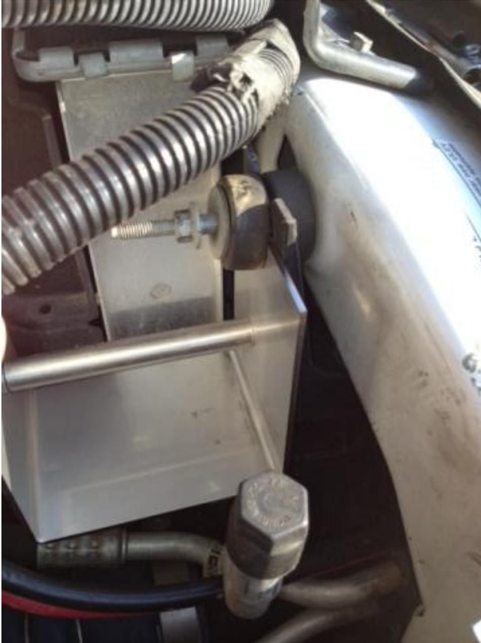
8. Place crossover hose over the fan shroud. You will then cut the 3/8" factory hose and remove approximately 1/2" from the length during the cut. This allows for the Tee assembly to be installed. Install small hose clamps supplied and tighten.
